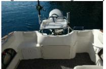
Batteries, oil tanks and wash down gear are all stowed under the transom moulding. The port side seat is removable to allow easy access over the transom.
