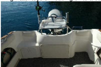
Batteries, oil tanks and wash down gear are all stowed under the transom moulding. The port side seat is removable to allow easy access over the transom.
